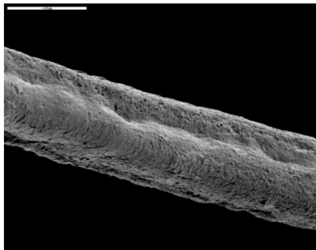
Figure 6 SEM for a CA/CB (55/45%) blend fiber treated with 0.5N SM/methanol. The scale bar represents 50 \mu\text{m} .
