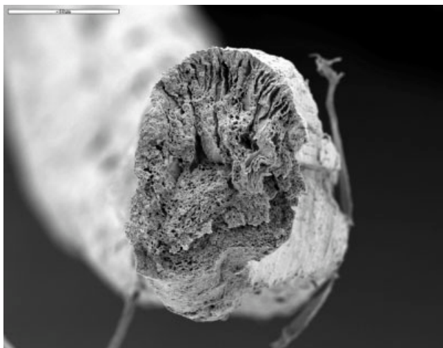
Figure 3 SEM for a CA/CB (55/45%) as-spun fiber blend. The scale bar represents 50 \mu\text{m} .
